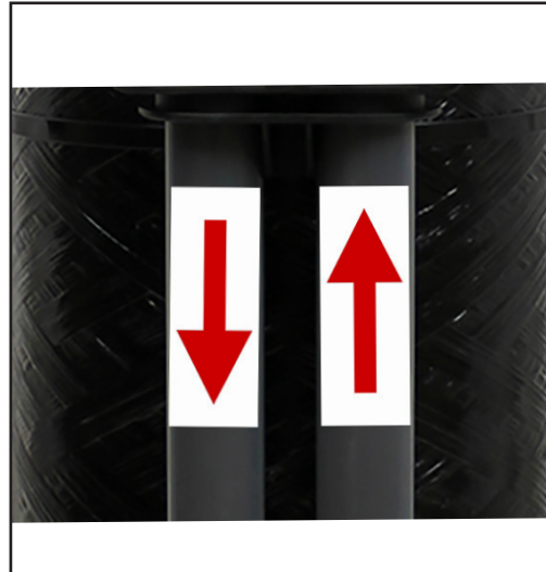
Take note of the water flow arrows and plumb in your incoming and outgoing water. Use Teflon tape only on connector threads. The use of other sealants can damage the threads.
