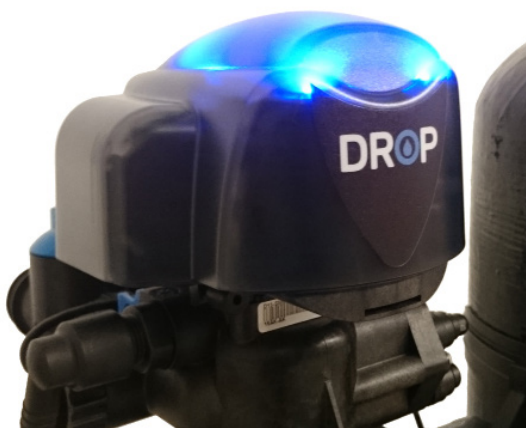
Image of DROP Treatment Valve Lights during Normal Operations.
